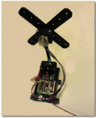
Reaction Wheel Pendulum
