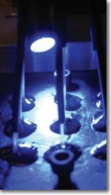
A fiber-optical array for medical research is being cured under ultraviolet light
