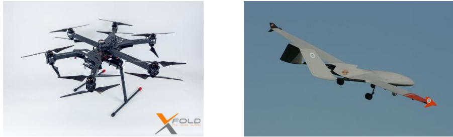
Figure 1. XFold Travel 12 multirotor (left) and the Oklahoma State University designed Talos UAV (right).
