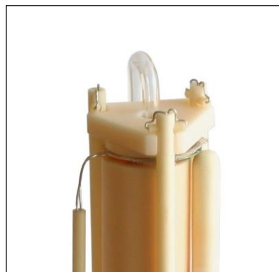
Figure 8-15: Fully assembled emf concentration cell with bent outer gas supply quartz tube mounted with triangular spring load assembly
