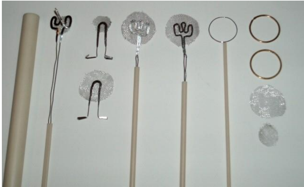
Figure 4-10. Alumina/Pt electrode contacts and Au gaskets typically supplied with a normal system in version A-6. From left: Multibore alumina gas supply tube (for use with 20 and 24 mm sample support tube) and INH2N12 inner two-wire electrode contact with net and “finger”. Two GP2N# general purpose electrode nets of different diameter with clip on to GP2 2-wire contacts. Two H2N# two-wire “hand” electrode contacts with net, GR# guard-ring/reference electrode contact, 2 gold gaskets for sealing, and 2 Pt# nets for general contact purposes.
