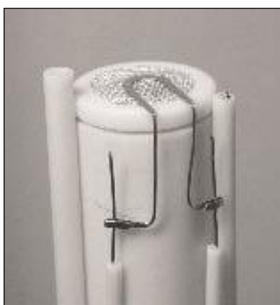
Figure 8-2: Support disk on support tube, with GP2N# as electrode connected by two GP1. This forms the lower electrode; the sample and another GP2N# are to be placed over it. Also showing outer gas supply tube (left) and control thermocouple TCC/D (right).
